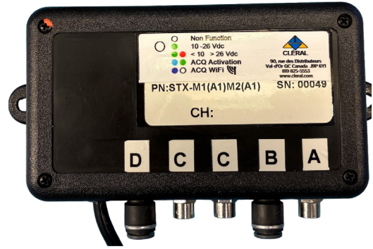
STX (Wi-Fi transmitter/receiver for air/mechanical sensors)
